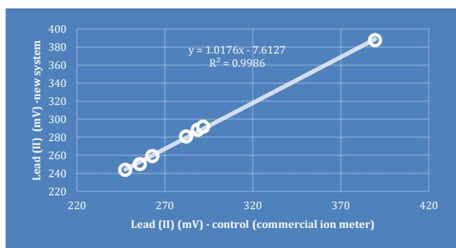
Fig. 4: Potentiometric measurement of lead (II) ions in water samples.
