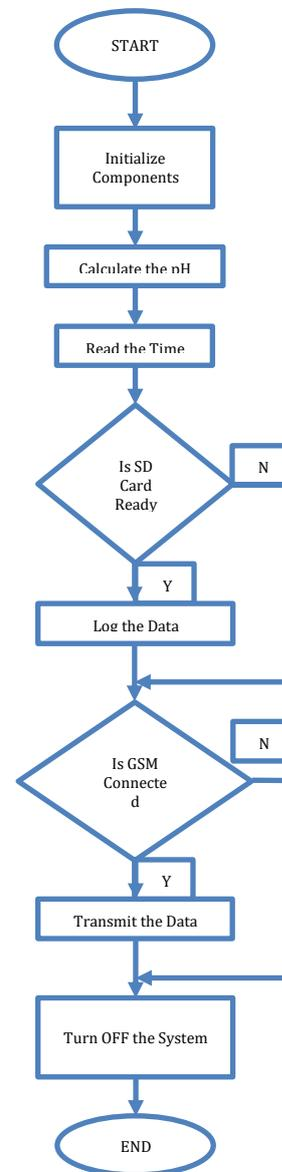
Fig. 3: Flowchart for reading the value.
